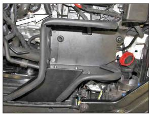
15. Install the heat shield assembly onto the mounting studs and secure the mounting bracket to the air filter housing with the provided hardware.
