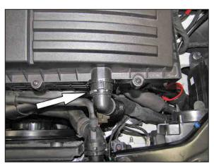
5. Disconnect the air injection hose from the upper air filter housing.
