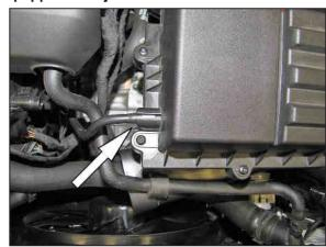
6. Disconnect the vacuum line from the air filter housing.
