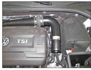
17. Install the secondary K&N® intake tube (27626) into the coupling hose at the turbo inlet and secure with the provided hose clamp.
