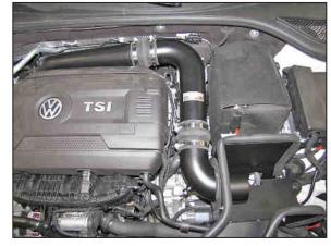
20. Install the primary intake tube onto the secondary tube and align with the mounting bracket installed onto the heat shield. Adjust the tubes for best fit and then secure with the provided hose clamps and hardware.
