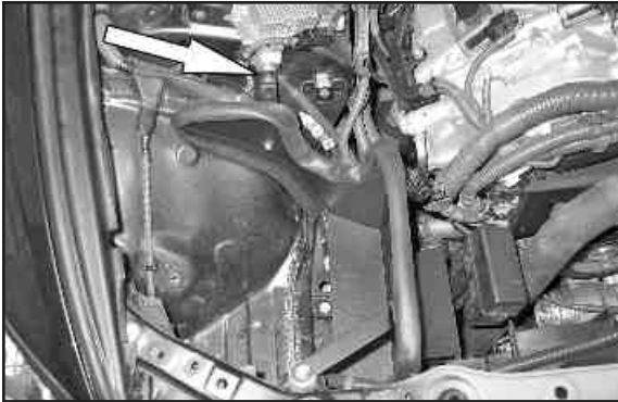
21. Set the heat shield into position and align with the rubber mounted stud, fender washer, and the ground strap bracket. Secure with provided hardware. NOTE: Be sure to use the provide spacer on top of the ground strap.
