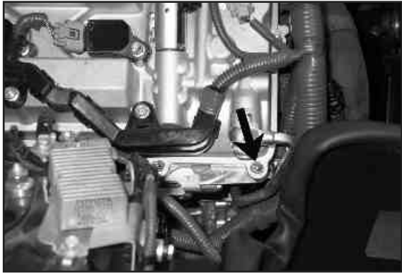
28. Remove the valve cover mounting bolt shown.
