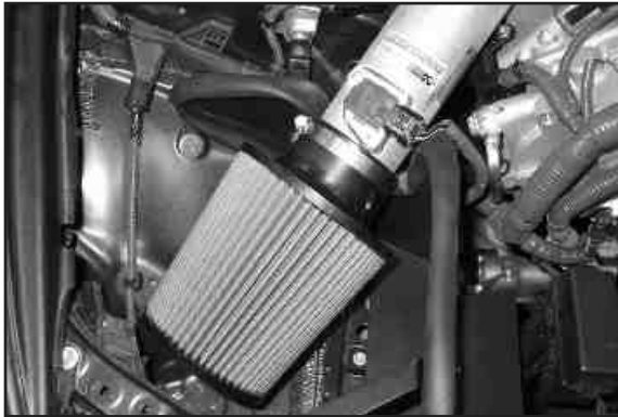
32. Install the K&N® air filter onto the intake tube and then tighten the hose clamp. NOTE: Drycharger® air filter wrap; part # RX-4990DK is available to purchase separately. To learn more about Drycharger® filter wraps or look up color availability please visit http://www.knfilters.com ®.
