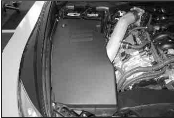
34. Reinstall the air filter cover and secure with the factory retainers.
