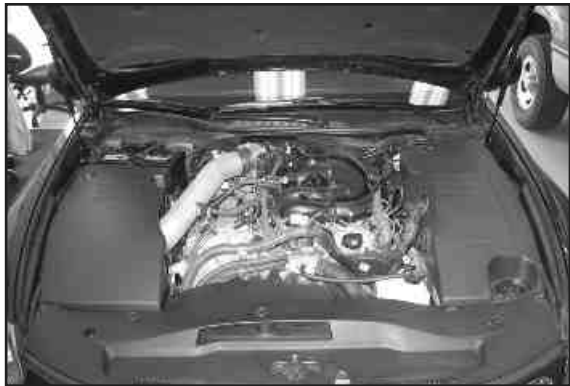
35. Reinstall the front cover and secure with the factory retainers.
