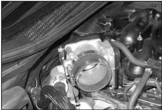
27. Install the silicone hose onto the throttle body and secure with the provided hose clamp.
