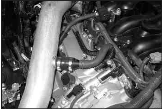
30. Reconnect the crank case vent hose to the fitting and secure with the factory hose clamp.
