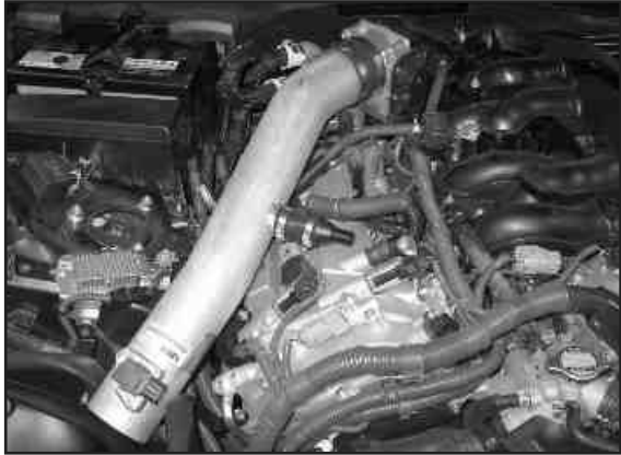
29. Install the K&N® intake tube into the silicone hose at the throttle body and align the bracket to the valve cover, secure with the factory valve cover bolt and hose clamp.
