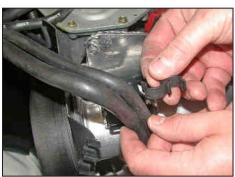
22. Remove the coolant hose clip as shown.
