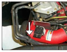
24. Secure the coolant hoses to the hose clip on the heatshield as shown.
