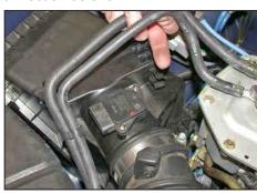
3. Unclip the coolant lines from the top of the air cleaner as shown.
