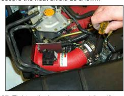
27. Tighten the hose clamp at the silicone hose as shown.
