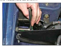
25. Using the bolt removed in step 10, secure the heat shield to the inner fender bracket but do not tighten at this time.
