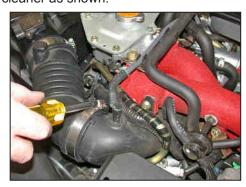
4. Loosen the hose clamp as shown.
