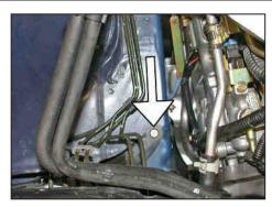
12. Install the stock air cleaner bolt into the original air cleaner mounting hole as shown.
