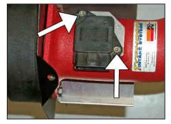
18. Install the mass air sensor from step 7 into the  $K\&N^{\tiny \circledcirc}$  intake tube and secure with the provided hardware as shown.
