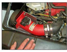
21. Install the complete assembly into the vehicle and slide the tube into the silicone hose as shown.
