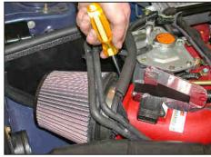
29. Install the K&N $^{\circ}$  air filter and and secure with the provided hose clamp as shown.
