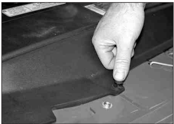
33. Reinstall the five radiator cover retaining clips removed in step #2.
