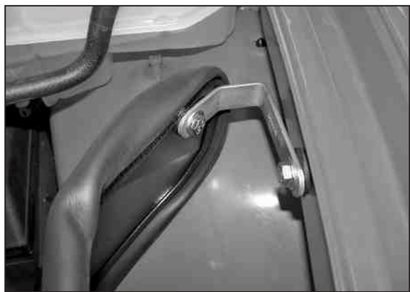
25. Install the heat shield bracket (#010077) onto the heat shield and inner fender and secure with the provided hardware.
