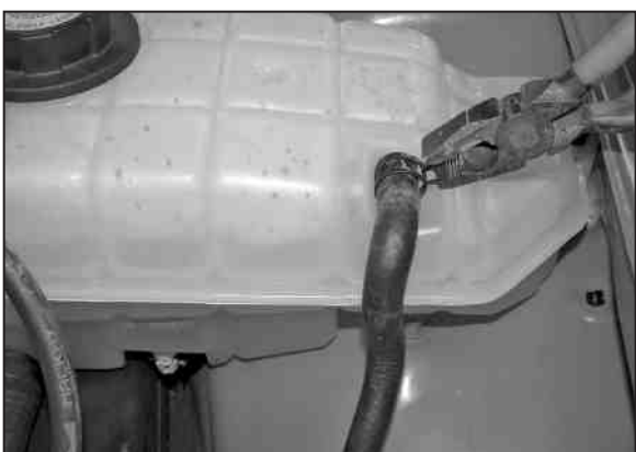
21. Make sure pressure is released from radiator cap before loosening spring clamp. Re-install the coolant reservoir back onto the two retaining studs, then, using a pair of pliers, loosen the spring clamp on the coolant reservoir hose. Rotate the coolant hose 90 degrees down as shown. Then resecure with the stock clamp.
