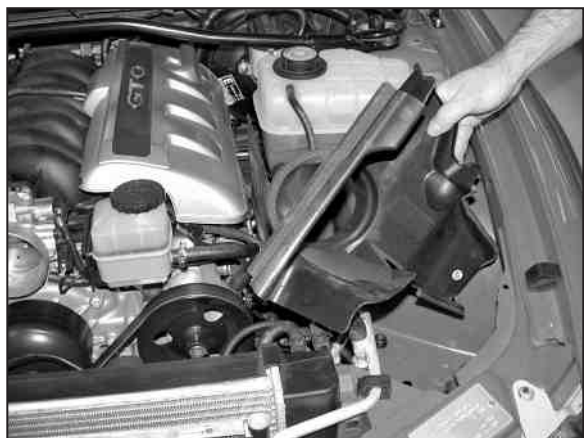
10. Lift up and pull out the air deflector from behind the head light.
