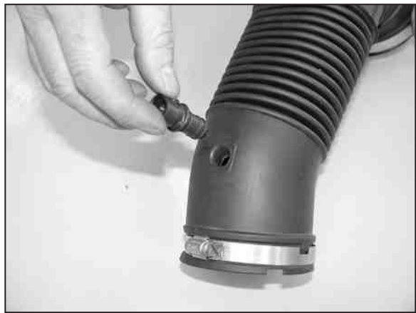
14. Remove the air temperature sensor from the stock intake tube.
