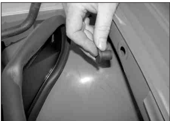
24. Install the threaded insert into inner fender as shown.
