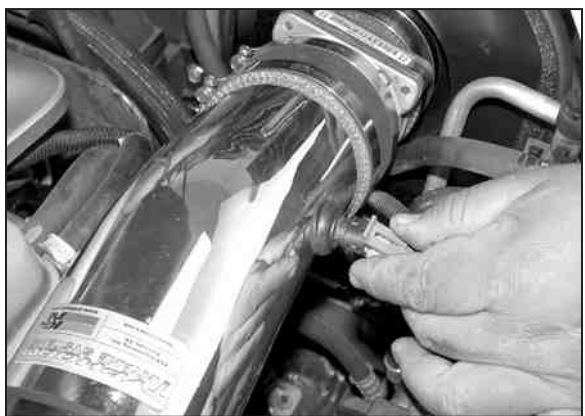
31. Reconnect the temperature sensor electrical connection.
