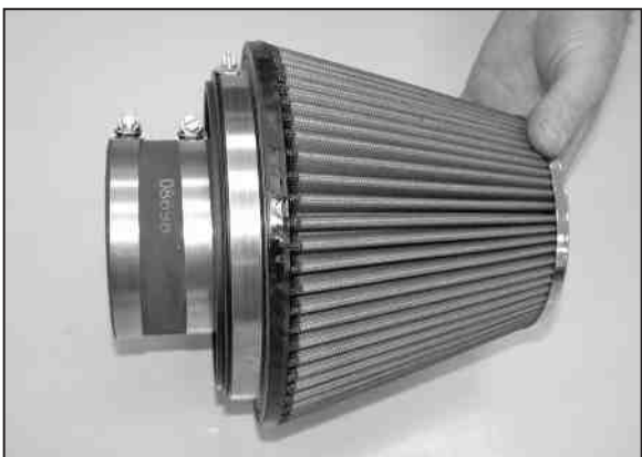
20. Install the provided silicone hose (08698) onto the filter adapter and secure with the provided hose clamp as shown.
