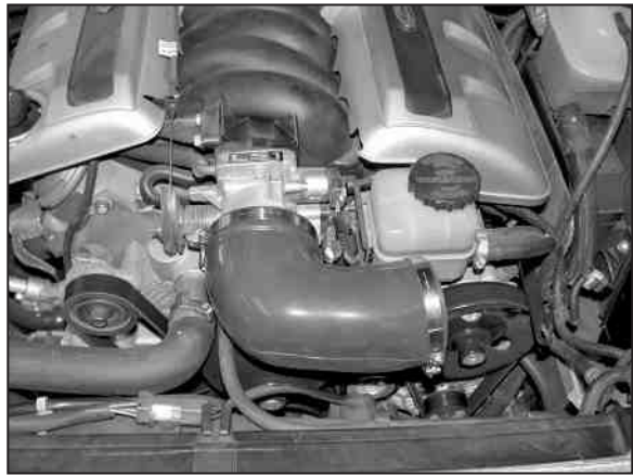
13. Install the silicone hose onto the throttle body and secure with the provided hose clamp.
