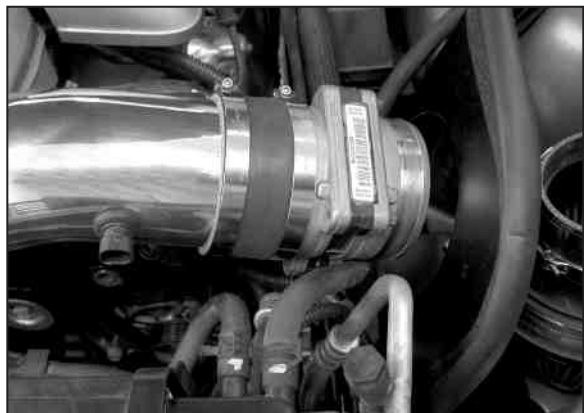
28. Install the mass air sensor assembly onto the K&N® intake tube and secure with the provided hose clamp.
