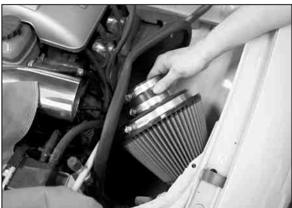
22. Set the heat shield assembly onto the inner fender, then set the filter charger assembly between the heat shield and fender as shown.
