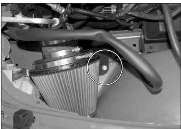
23. Secure the heat shield to the inner fender with the 6mm bolt provided. NOTE: Thread the 6mm bolt into the hole vacated in step #11.
