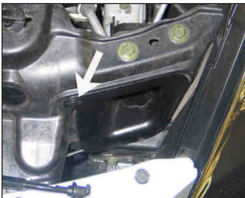
34. Re-install the driver's side fresh air duct and retaining clip.
