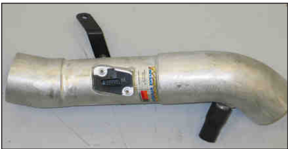
24. Install the mass air sensor into the K&N® intake tube and secure with the provided hardware.
