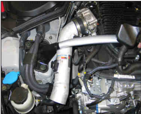
26. Install the intake tube assembly into the silicone hose at the throttle body and align the mounting bracket with the rubber mounted stud installed in step #14. Secure the intake tube with the provided hose clamp and hardware.
