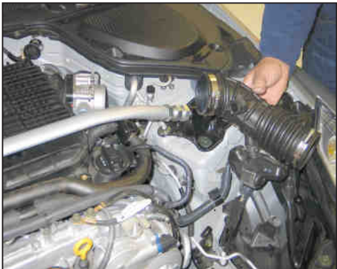
38. Release the spring clamp that secures the crankcase vent chamber to the intake tube. Then, remove the driver's side intake tube as shown.
