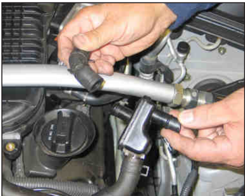
39. Disconnect the crankcase vent chamber hose from the engine valve cover, then from the crankcase vent chamber as shown.
