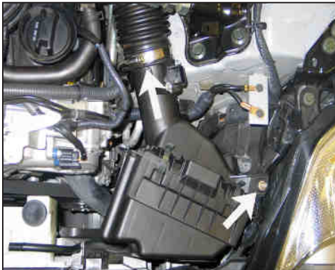
32. Loosen the hose clamp that secures the driver's side intake tube to the airbox. Then, remove the bolt that secures the driver's side airbox to the inner fender.
