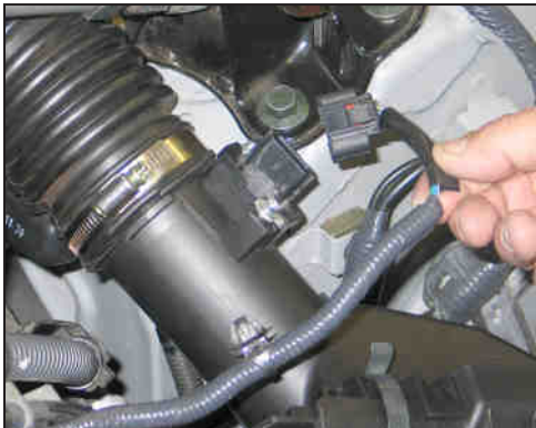
30. Unhook the driver's side mass air sensor wiring harness from the airbox, then disconnect the mass air sensor electrical connection as shown.
