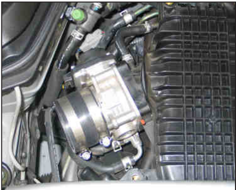
25. Install silicone hose (#08440) onto the throttle body and secure with the provided hose clamp as shown.
