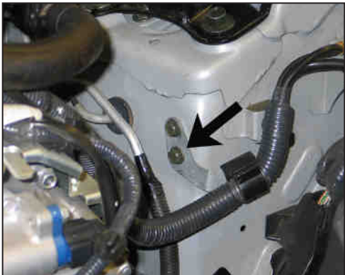
40. Remove the lower ground strap mounting bracket bolt shown.
