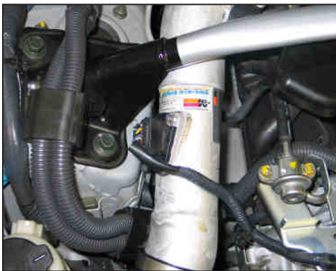
29. Re-connect the mass air sensor electrical connection.
