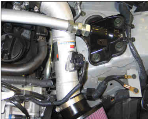
57. Re-connect the mass air sensor electrical connection.
