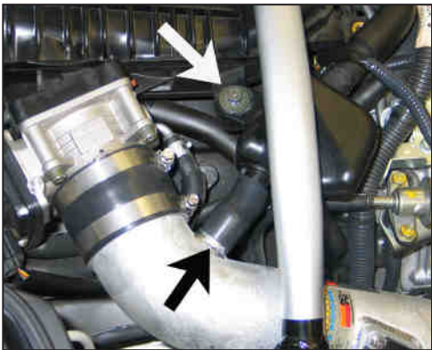
27. Install the crankcase vent chamber into the silicone hose attached to the vent tube of the K&N® intake tube. Secure the vent chamber with the bolt removed in step #10.
