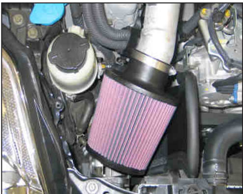
28. Install the K&N® air filter and secure with the provided hose clamp. NOTE: Drycharger® air filter wrap; part # RX-4990DK is available to purchase separately. To learn more about Drycharger® filter wraps or look up color availability please visit http://www.knfilters.com ®.
