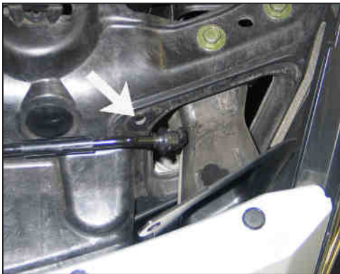
31. Remove the driver's side fresh air duct retaining clip. Slide the fresh air duct forward to disengage it from the driver's side airbox.
