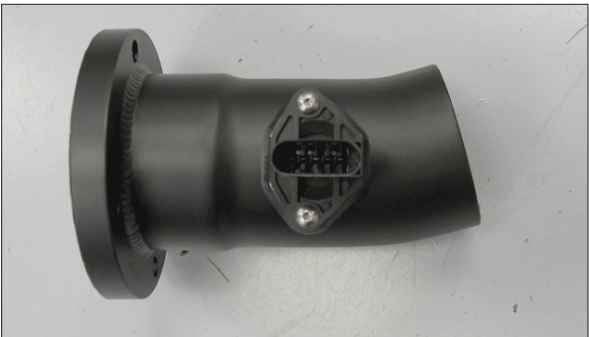
34. Install the mass air sensor into the left intake tube (27283) and secure with the provided hardware.
