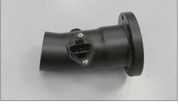
24. Install the mass air sensor into the right intake tube (27284-1) and secure with the provided hardware.
