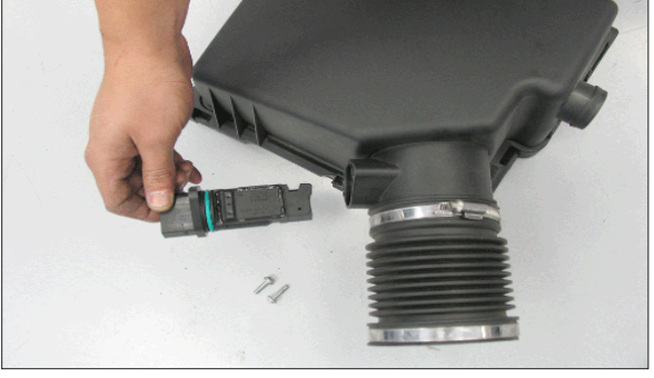
23. Remove the two screws that secure the mass air sensor to the right upper air box and then remove the mass air sensor as shown.
