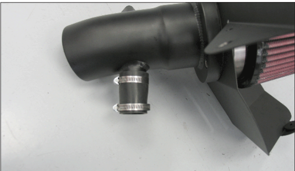
27. Install the provided air injection hose onto the intake tube and secure with the provided hose clamp as shown.
