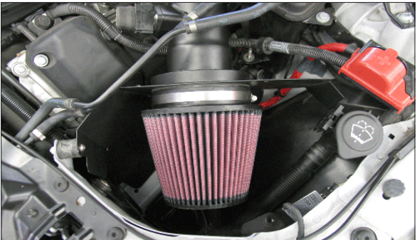
38. Install the air filter and secure with the provided hose clamp.
