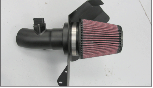
26. Install the air filter onto the filter adapter and secure with the provided hose clamp.
