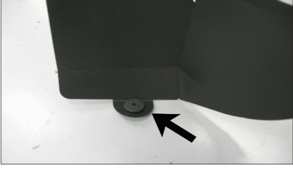
19. Install the provided grommets into the 11/16" id holes in the bottom of the heat shield as shown.
