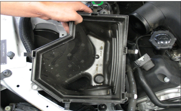
12. Remove the right lower air box from the vehicle.
