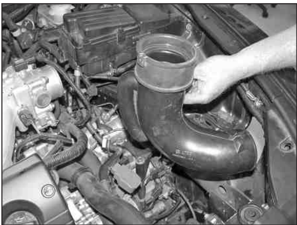
23. Remove the air inlet duct as shown.
