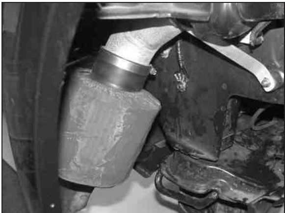
42. From underneath the vehicle install the K&N® air filter onto the cold air tube and secure with the provided hose clamp as shown.
