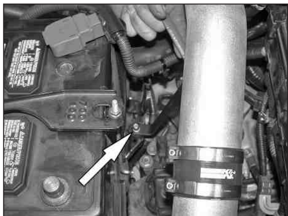
39. Tighten the hardware on the “Z” bracket at the tube and at the rubber mounted stud as shown.
