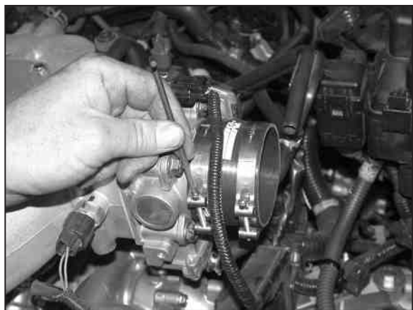
25. Install the silicone hose and hose clamps and tighten the hose clamp on the throttle body.
