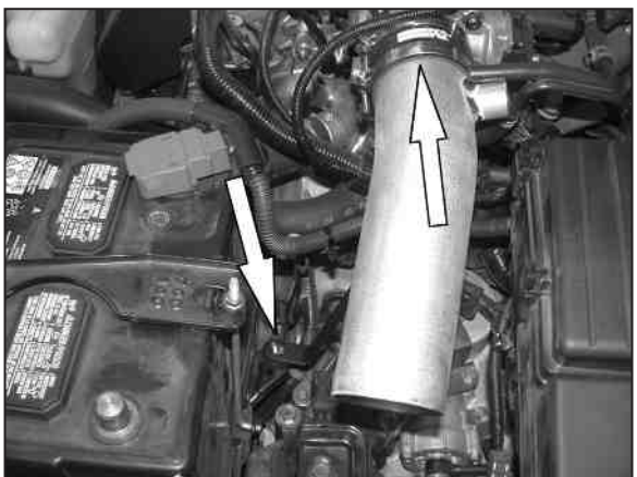
29. Slide the K&N short ram tube into the silicone hose on the throttle body, then, line up the "Z" bracket with the rubber mounted stud from step 26.
