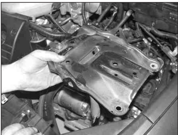
21. Remove the battery tray as shown.
