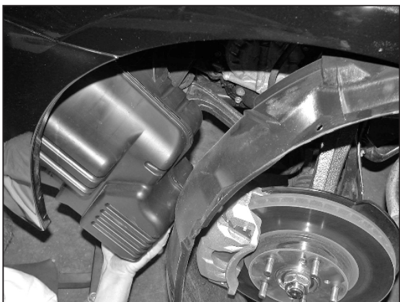
14. Remove the air intake resonator as shown. NOTE: Not all air intake resonators may look the same. NOTE: On '04-'06 models, skip steps 15 thru 24 and proceed to step 25.
