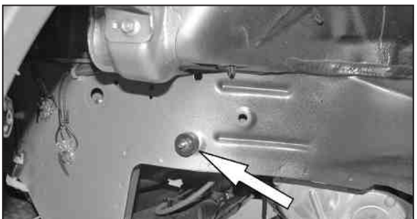
33. Install the rubber mounted stud into the original resonator mounting hole from step 13. NOTE: On '04 models, install the rubber mounted stud into threaded hole as shown.
