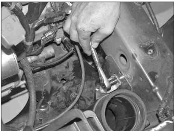
22. Loosen and remove the bolt that secures the air inlet duct to the inner fender as shown.
