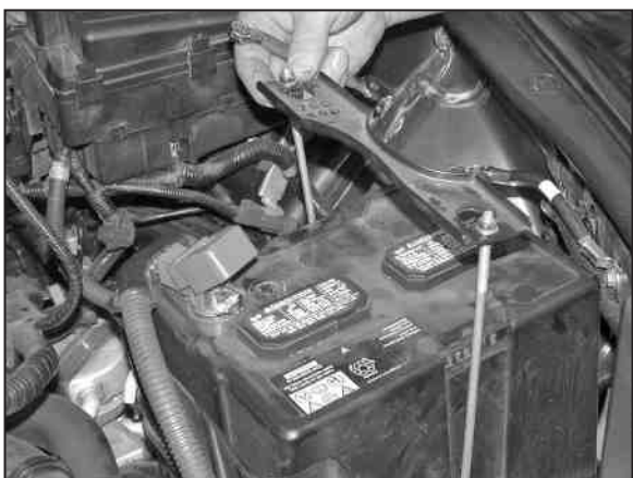
17. Loosen and remove the battery hold down bracket as shown.
