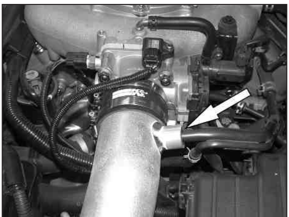
30. Slide the crankcase vent hard line into the vent on the K&N short ram tube as shown.
