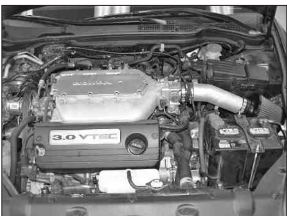
45. This K&N® high flow intake system has been designed to be used in two different configurations. In the case of inclement weather, the cold air tube can be removed and the air filter can be clamped onto the intake tube located in the engine compartment to avoid the possibility of ingesting water into the engine.
