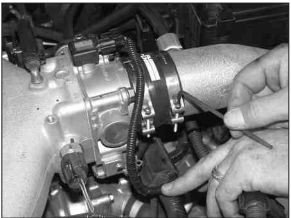
38. Tighten the hose clamp at the throttle body.
