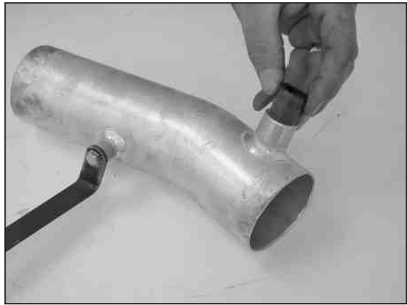
28. Slide the provided silicone hose into the vent on the K&N short ram tube.
