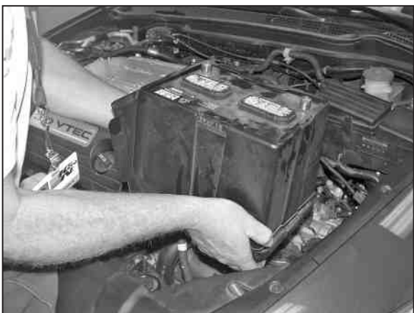
19. Remove the battery and the plastic cover as shown.
