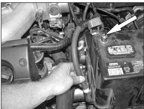
18. Disconnect the positive battery cable and unclip the cable from the side of the plastic battery cover.
