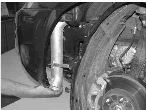
34. Slide the K&N cold air tube into the vehicle from underneath the vehicle as shown. NOTE: Before installing the intake tube, inspect the inside of the tube for any debris, then clean the inside out with water and a towel. Inspect the tube one more time before proceeding to the next step.
