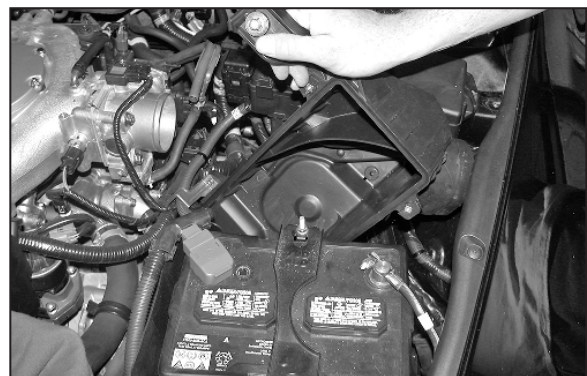
10. Pull up to release the lower air cleaner assembly from the stock air inlet duct and remove as shown. NOTE: K&N Engineering, Inc., recommends that customers do not discard factory air intake.
