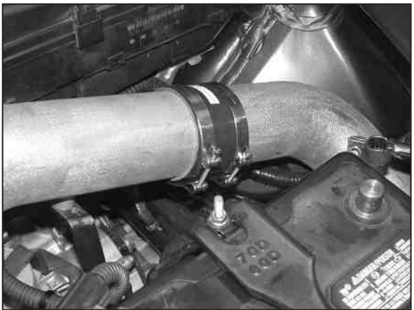
36. Slide the silicone hose located on the short ram tube onto the cold air tube as shown.
