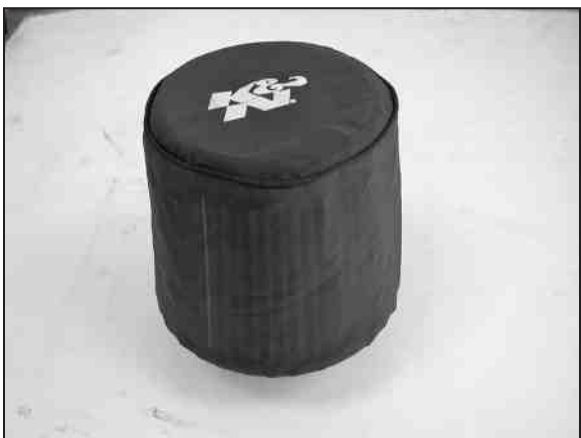
41. Slide the provided K&N® Drycharger® onto the K&N® air filter as shown.
