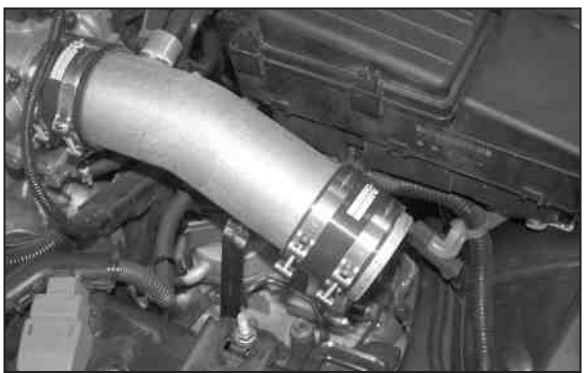
32. Slide the silicone hose and hose clamps onto the K&N short ram tube as shown. NOTE: Slide the silicone hose past the edge of the tube as this will help with the installation of the cold air tube.
