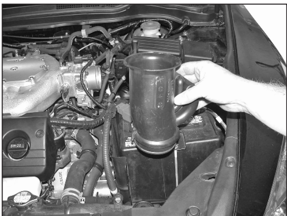
16. Remove the air inlet duct as shown.
