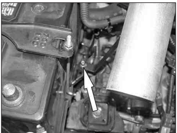
31. Secure the "Z" bracket to the rubber mounted stud using the provided hardware as shown, but do not tighten completely as this time.
