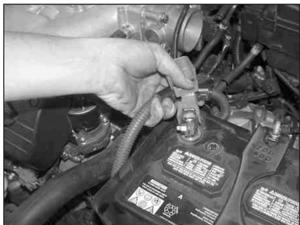
24. Reverse the removal process and reinstall the battery tray, battery, plastic cover, battery hold down bracket, and the positive battery cable as shown.
