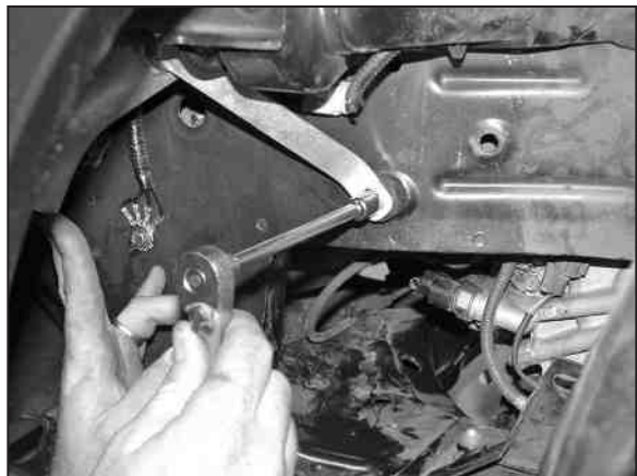
40. Tighten the hardware on the rubber mounted stud that secures the cold air tube as shown.
