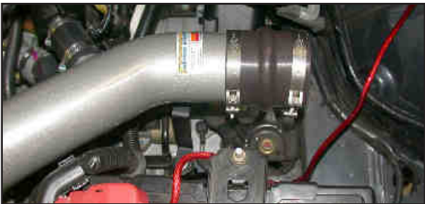
25. Install the silicone hump hose and hose clamps onto the K&N® short ram tube as shown.
