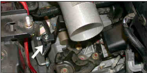
20. Line up the bracket with the rubber mounted stud and secure with the provided hardware but do not tighten at this time.
