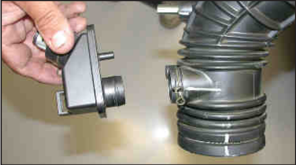
15. Remove the crankcase vent chamber from the stock intake tube as shown.
