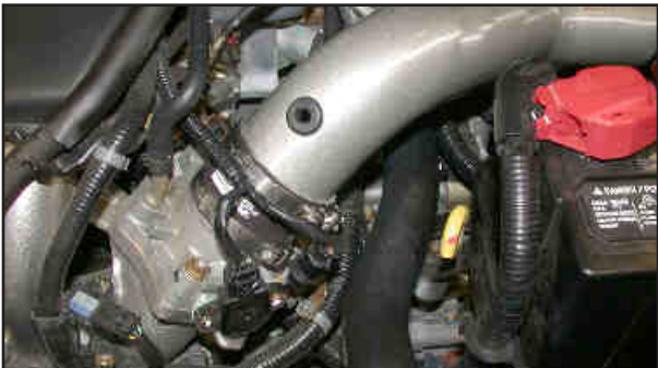
19. Slide the K&N® short ram intake tube into the silicone hose as shown.
