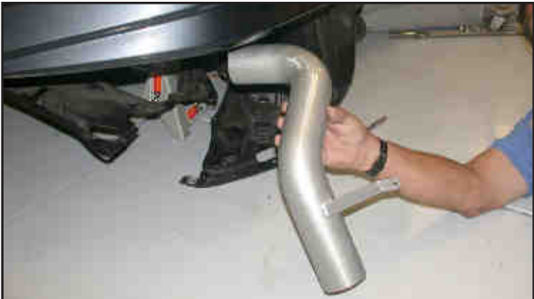
27. Install the K&N® cold air tube from underneath the vehicle as shown.
