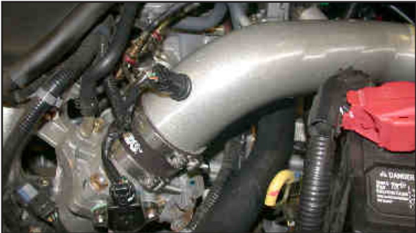
21. Install the air temperature sensor into the grommet as shown.
