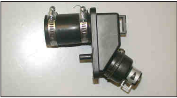
23. Install the provided hose and hose clamps onto the stock crankcase vent chamber as shown.
