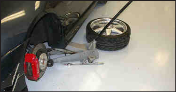
11. Raise the vehicle up and support it with jack stands, then, remove the front tire as shown.
