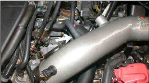
22. Reconnect the vent hose to the vent on the K&N® short ram tube as shown.
