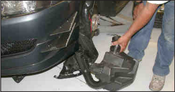
13. Remove the two bolts that secure the resonator to the inner fender, then, remove the resonator as shown.
