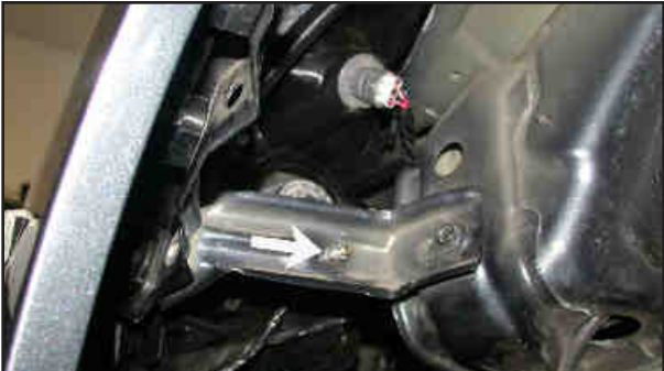
26. Install the provided rubber mounted stud onto the front of the fender brace and secure with the provided hardware as shown.
