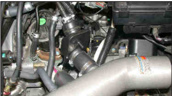
24. Install the crankcase vent chamber onto the vent on the K&N® short ram tube, then, connect the other end to the crankcase vent hard line as shown
