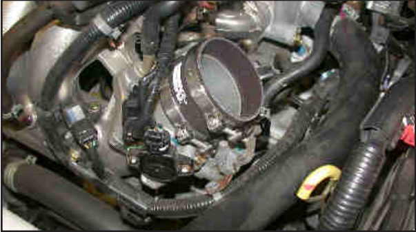
14. Install the silicone hose and hose clamps onto the throttle body and tighten as shown.
