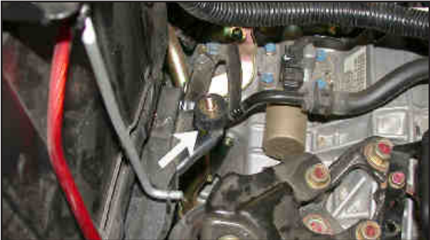
16. Install the rubber mounted stud into the original air cleaner mount as shown.
