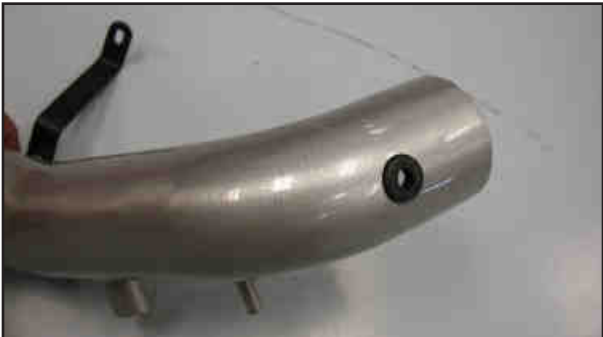
18. Install the provided grommet into the hole on the K&N® short ram tube as shown.
