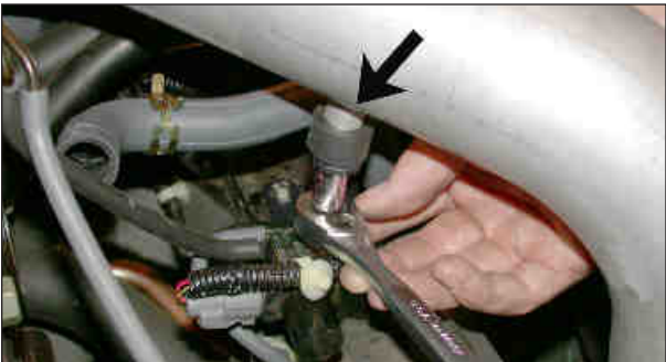
31. Using the provided hardware secure the "Z" bracket to the rubber mounted stud as shown.
