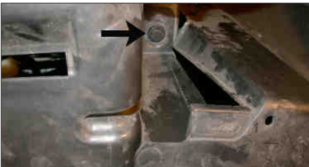
36. Remove the two remaining push clips located on both sides of the inner wheel house as shown.
