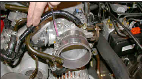
26. Install the silicone step hose and hose clamps onto the throttle body and tighten as shown.
