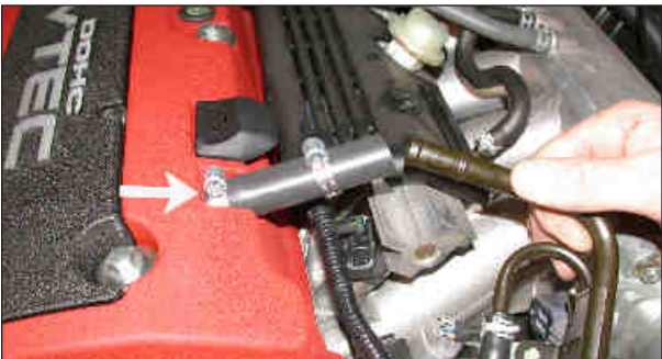
14. Install the provided silicone hose and hose clamps onto the crank case vent on the cam cover as shown.
