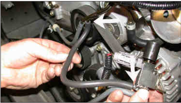
21. Using the remaining piece of 4mm hose from step 16, trim a 7-1/2" length of hose and reconnect the hard line to the upper port on the solenoid as shown.
