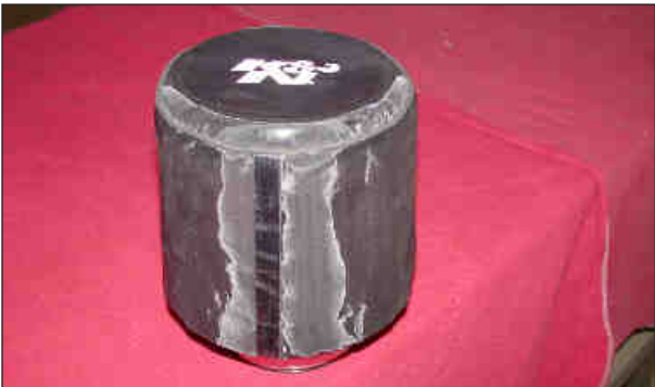
42. Install the K&N® Drycharger® onto the K&N® X-Stream® air filter as shown. NOTE: Please be aware the Drycharger® is water repellent, not water proof. Depending on conditions and usage the water repellent treatment is good for 1 to 2 years. See the parts list to reorder a new Drycharger® if necessary.
