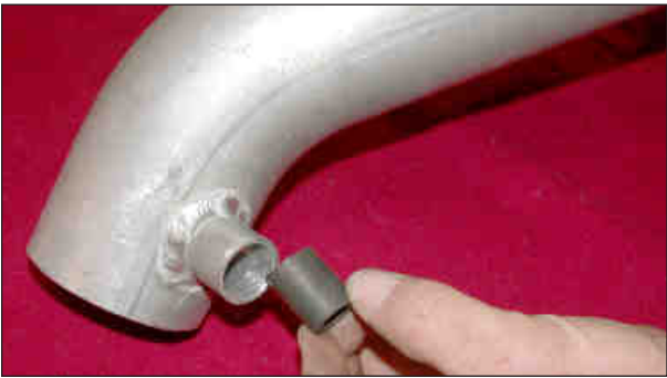
27. Install the provided 1" length of hose into the vent on the end of the K&N® intake tube as shown. NOTE: Before installing the provided hose, inspect the inside of the tube for any debris, then clean the inside out with water and a towel. Inspect the tube one more time before proceeding to the next step.
