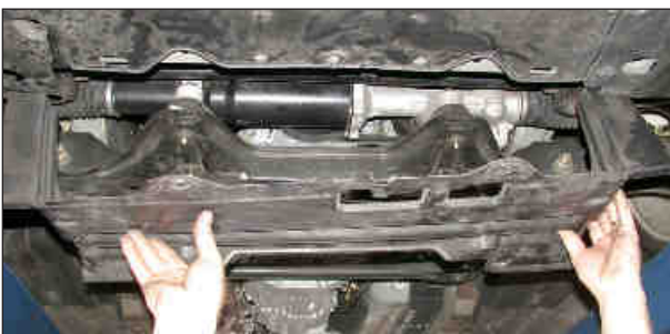
37. Remove the splashguard as shown.
