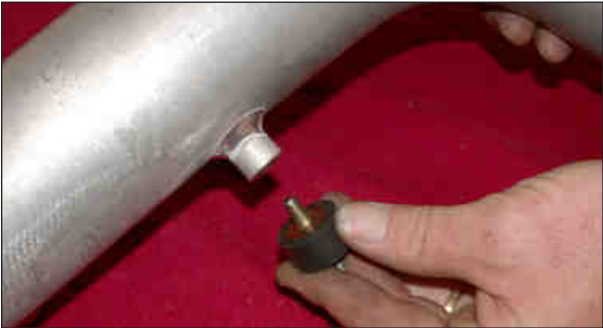
28. Install the rubber mounted stud into the threaded boss on the K&N® intake tube as shown.
