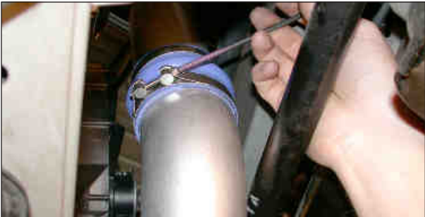
41. Tighten the hose clamp on the silicone hump hose as shown.
