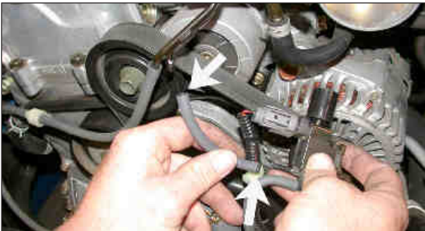
18. Disconnect the vacuum hose from the upper solenoid port and from the hard line as shown.
