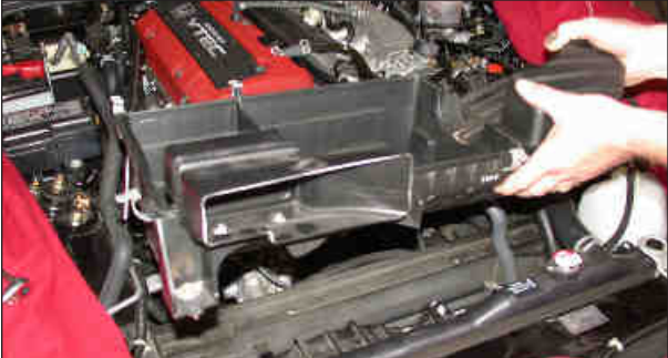
10. Remove the lower air cleaner assembly as shown. NOTE: K&N Engineering, Inc., recommends that customers do not discard factory air intake.
