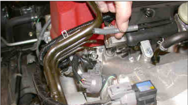
13. Remove the vacuum hose from the lower hard line as shown.
