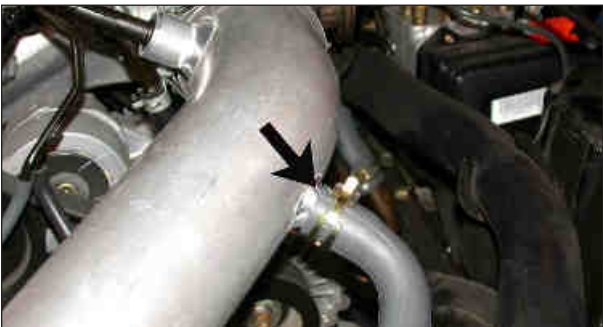
32. Reconnect the stock air injection pump hose to the K&N® intake tube as shown.
