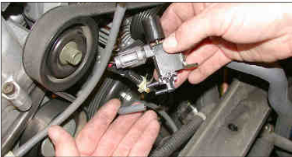
19. Disconnect the vacuum hose from the lower solenoid port as shown.
