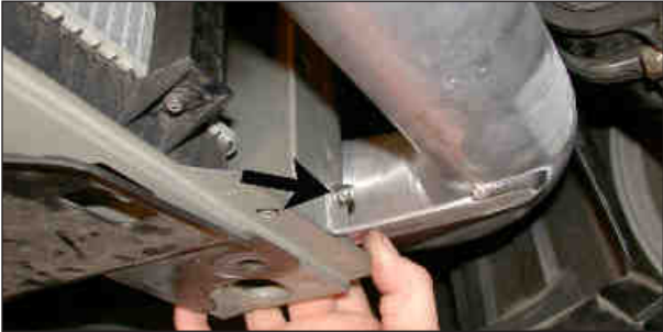
40. Secure the bracket to the core support using the provided hardware.
