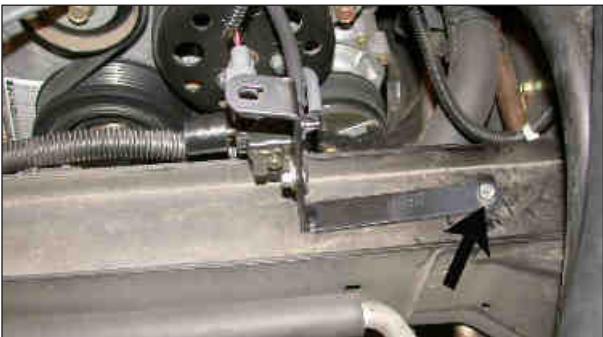
25. Using the provided hardware secure the "Z" bracket to the original air cleaner mounting location as shown.
