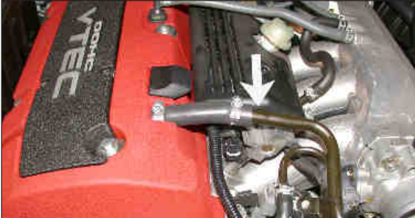
17. Reconnect the crank case vent hard line as shown.
