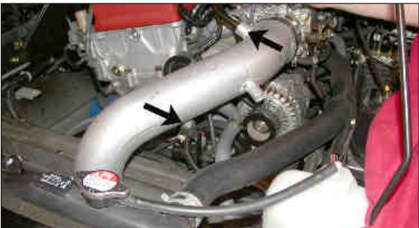
30. Slide the K&N® intake tube into the silicone hose on the throttle body, then, slide the crank case vent hard line into the vent on the intake tube as shown. Before tightening the silicone hose, line up the rubber mounted stud with the "Z" bracket as shown.
