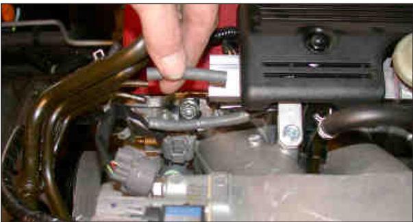
12. Remove the vacuum hose from the upper hard line as shown.
