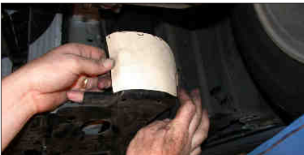
38. Using the provided template, use a white paint pen and mark the trim lines on the inner fender valance, then cut with an appropriate air or hand tool.
