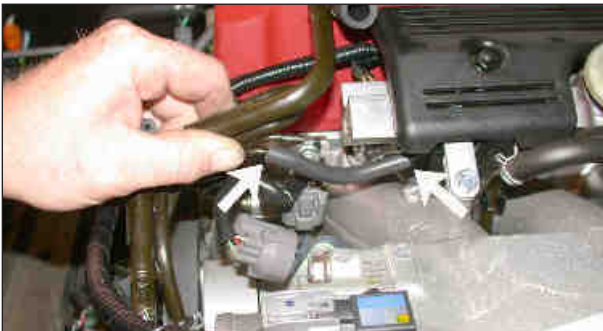
15. Using the provided 18" length of 4mm hose, trim a 3-1/2" length of hose and reconnect the lower hard lines as shown.
