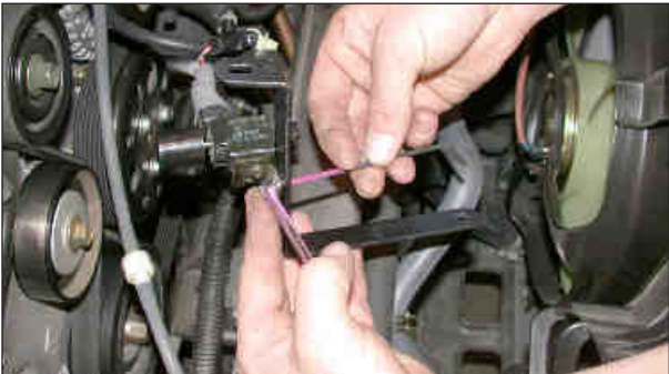
24. Using the provided hardware secure the solenoid to the provided "Z" bracket as shown.
