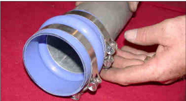
29. Install the silicone hump hose and hose clamps onto the K&N® intake tube as shown.
