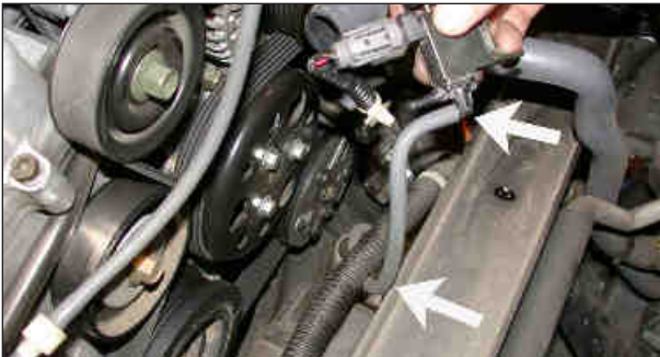
20. Reroute the vacuum hose behind the wire harness, then, reconnect the vacuum hose to the lower solenoid port as shown.
