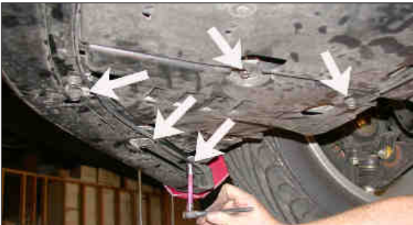
34. Remove the five bolts that secure the lower valance as shown.
