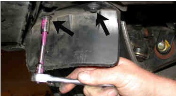
33. Raise the vehicle up and support it with jack stands, then, remove the rock guard from the lower right side valance located in front of the front tire as shown.
