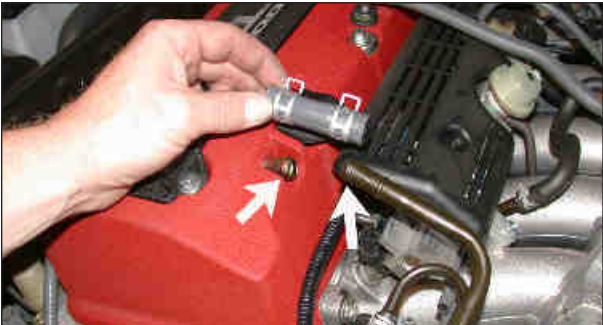
11. Remove the stock rubber hose from the crank case vent on the cam cover and from the hard line as shown.
