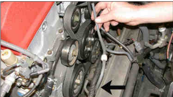
23. Reroute the vacuum hose behind the wire harness, then, reconnect the vacuum hose to the hard line as shown.
