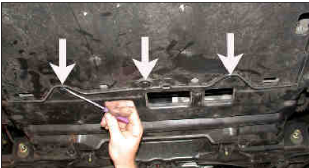
35. Remove the 5 push clips that secure the underbody splash guard as shown.
