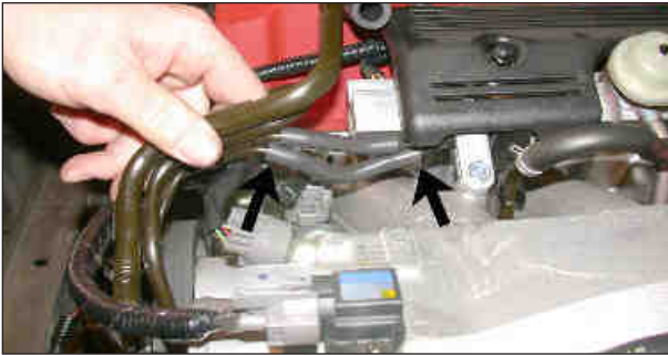
16. Using the remaining piece of 4mm hose from step 15, trim a 2-1/2" length of hose and reconnect the upper hard lines as shown.
