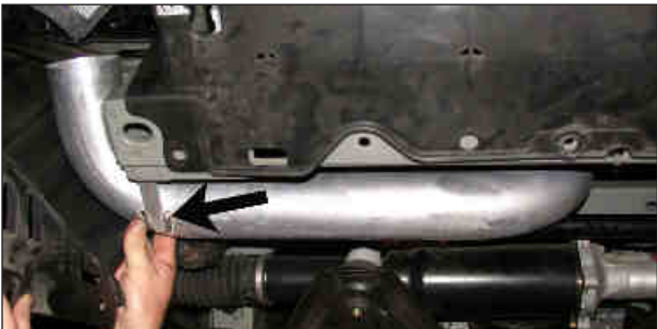
39. Slide the K&N® cold air tube into the silicone hose, then, line up the bracket with the radiator core support as shown. NOTE: Before installing the cold air tube, inspect the inside of the tube for any debris, then clean the inside out with water and a towel. Inspect the tube one more time before proceeding to the next step.
