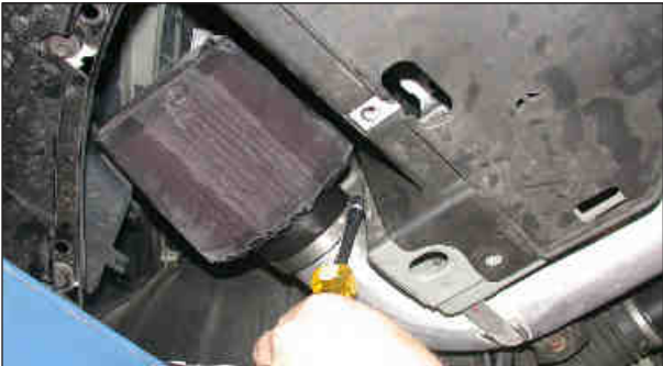
43. Install the K&N® X-Stream® air filter onto the K&N® cold air intake tube and tighten as shown.
