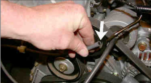
22. Disconnect the vacuum hose from the hard line as shown.
