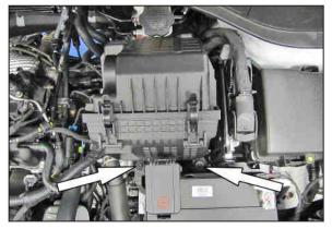
8. Remove the two bolts that secure the air filter housing and then remove the air filter housing from the vehicle.
