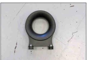
10. Install the filter adapter onto the mounting bracket and secure using the provided hardware. NOTE: The bracket part number will be covered over by the filter adapter when it is installed on the correct side of the bracket.
