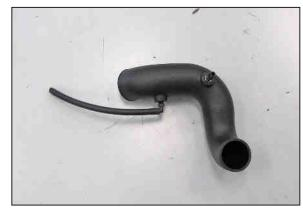
22. Install the provided vent hose onto the 90° vent fitting as shown.
