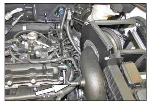
24. Connect the factory crank case vent hose to the fitting installed into the K&N<sup>®</sup> intake tube and then connect the EVAP hose to the factory valve.
