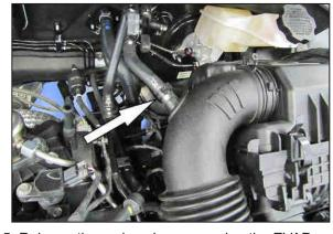
5. Release the spring clamp securing the EVAP vent hose to the valve and then disconnect the hose from the valve.
