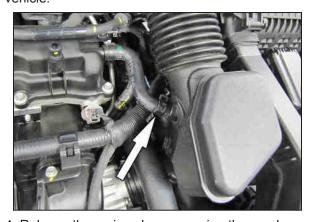
4. Release the spring clamp securing the crank case vent hose to the intake tube and then disconnect the crank case vent hose from the intake tube.
