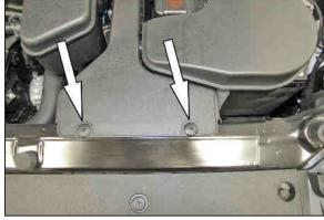
3. Remove the two plastic retaining screws and then remove the fresh air intake duct from the vehicle.
