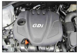
2. Lift up and remove the decorative engine cover from the engine.
