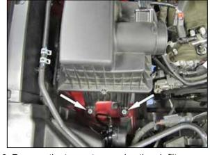
6. Remove the two nuts securing the air filter housing to the inner fender and then remove the housing from the vehicle.
