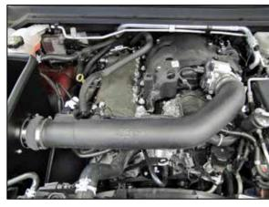
18. Install the provided hump coupler (08699) onto the K&N® intake tube, then install the intake tube assembly into the coupler at the throttle body and align with the filter adapter. Slide the hump coupler onto the filter adapter, adjust the tube for best fit and secure with the provided hose clamps.
