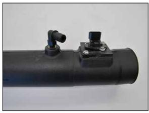
16. Install the 90° vent fitting into the K&N® intake tube as shown.
