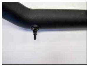
17. Install the quick connect fitting into the K&N<sup>®</sup> intake tube as shown.
