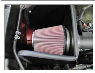
21. Install the K&N® air filter onto the filter adapter and secure with the provided hose clamp. NOTE: Drycharger® air filter wrap; part # RF-1042DK is available to purchase separately. To learn more about Drycharger® filter wraps or look up color availability please visit http://www.knfilters.com®.
