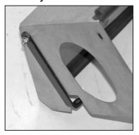
13. Install the provided "L" bracket #070026 onto the heat shield with the provided hardware as shown.
