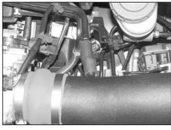
23. Install the provided silicone vent hose onto the K&N® intake tube and then install the crankcase vent tube into the silicone hose as shown.
