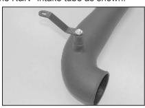
19. Install the tube mount bracket # 070065 onto the  $K\&N^{\circ}$  intake tube as shown.
