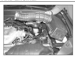
8. Remove the airbox lid and intake tube as shown.
