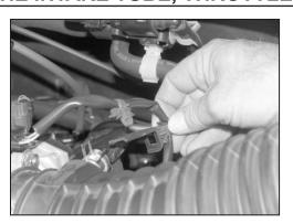
4. Unhook the wiring harness retaining clips as shown.
