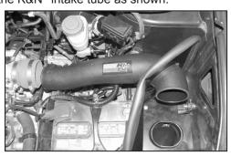
20. Set the K&N® intake tube in place through the heat shield but not onto the throttle body as shown.
