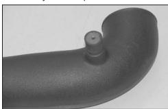
18. Install the provided rubber mounted stud onto the K&N® intake tube as shown.
