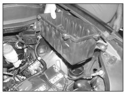
10. Remove the lower airbox housing as shown. NOTE: K&N Engineering, Inc., recommends that customers do not discard factory air intake.
