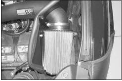
21. Install the air filter onto the K&N<sup>®</sup> intake tube and secure with the provided hose clamp.
