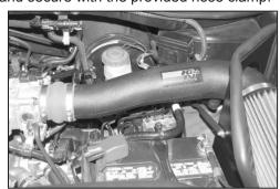
22. Install the K&N® intake tube into the silicone hose at the throttle body and align the mounting bracket with the heat shield bracket and mounting tab on the strut tower. Tighten the hose clamp and secure the bracket to the heat shield bracket and mounting tab on the strut tower with the provided hardware.
