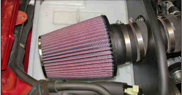
23. Install the K&N® air filter onto K&N® intake tube and secure with the provided hose clamp. NOTE: Drycharger® air filter wrap; part # RF-1032DK is available to purchase separately. To learn more about Drycharger® filter wraps or look up color availability please visit http://www.knfilters.com ®.
