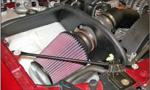
24. Re-install the core support brace removed in step #4 with the stock hardware. NOTE: Adjust the air filter and intake tube at this time for minimum of 1/2" clearance then tighten the hose clamps.
