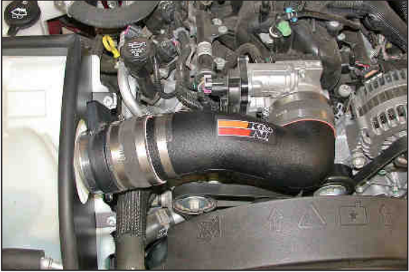
20. Install the K&N® intake tube assembly into the silicone hose at the throttle body and onto the saddle clamp as shown, then secure with the provided hose clamps.
