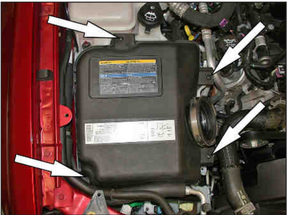
6. Loosen and remove the four screws that secure the upper air box lid.
