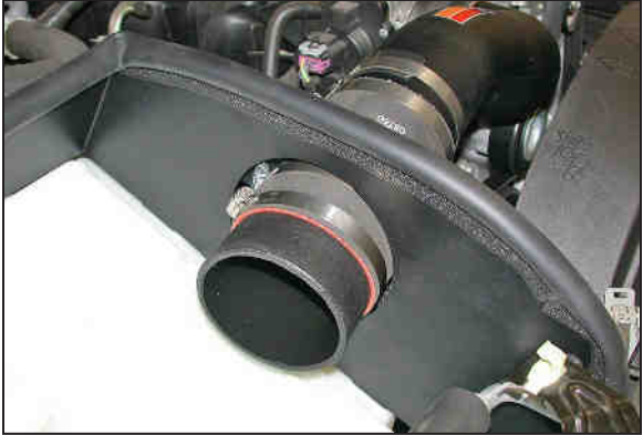
22. Install the "EH" tube assembly onto the mass air sensor and secure with the provided hose clamp.
