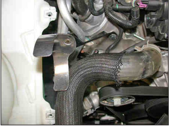
13. Install the tube bracket assembly onto the engine using the hardware provided. NOTE: The supplied bolt threads into the threaded hole in the engine vacated by the wire harness clip in step #11.
