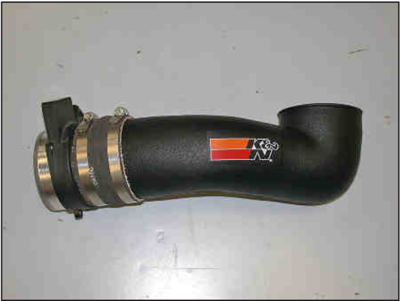
19. Install the mass air sensor assembly onto the K&N intake tube (EI) as shown. NOTE: Do not completely tighten at this time.
