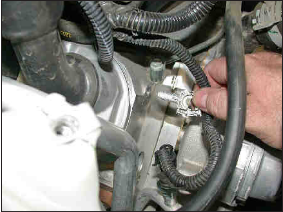
11. Unthread the retaining clip from the engine as shown.
