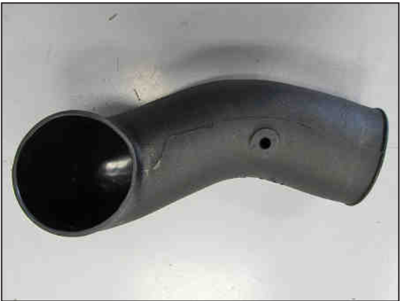
18b. Install the provided grommet into the hole drilled into the intake tube in step #18a.
