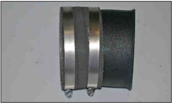
21. Install the supplied silicone hose (08625) onto the small diameter end of the "EH" K&N® intake tube.
