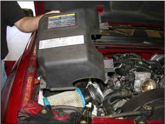
7. Remove the upper air box lid from the vehicle as shown.
