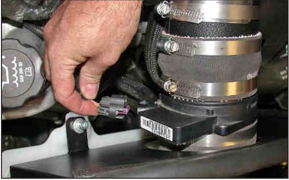
25. Reconnect the mass air sensor electrical connection as shown.
