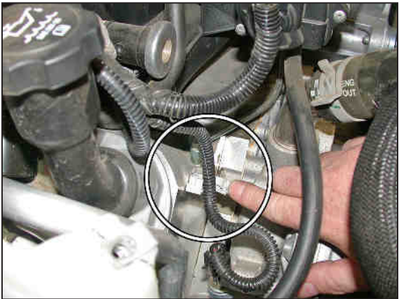
10. Using a screwdriver unlock the wiring harness from the retaining clip attached to the engine as shown.
