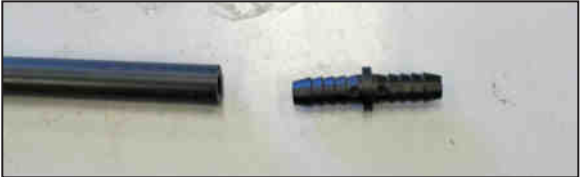
20a. On vehicles equipped with a crank case vent hose, install the supplied hose mender into the supplied crank case vent hose fitting.
