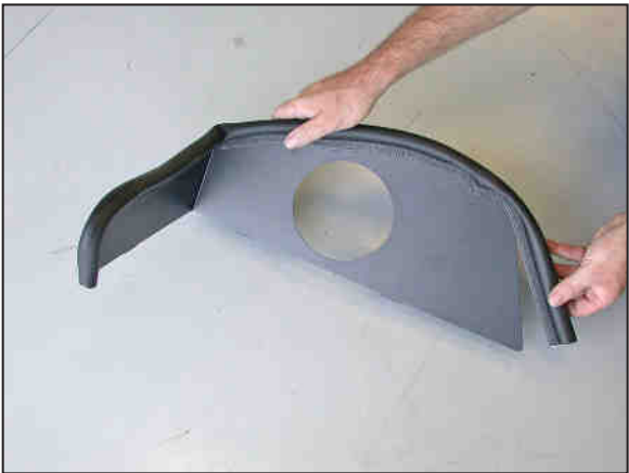
15. Install the provided edge trim onto the heat shield as shown. NOTE: Some trimming may be necessary.
