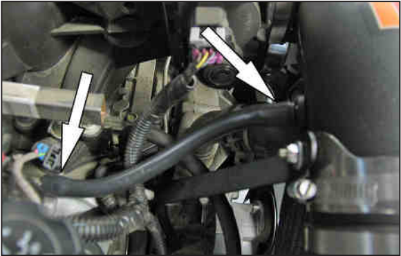
20b. Install the crank case vent assembly onto the valve cover fitting and then into the grommet installed into the K&N® intake tube as shown. NOTE: Some trimming of the vent hose will be necessary.
